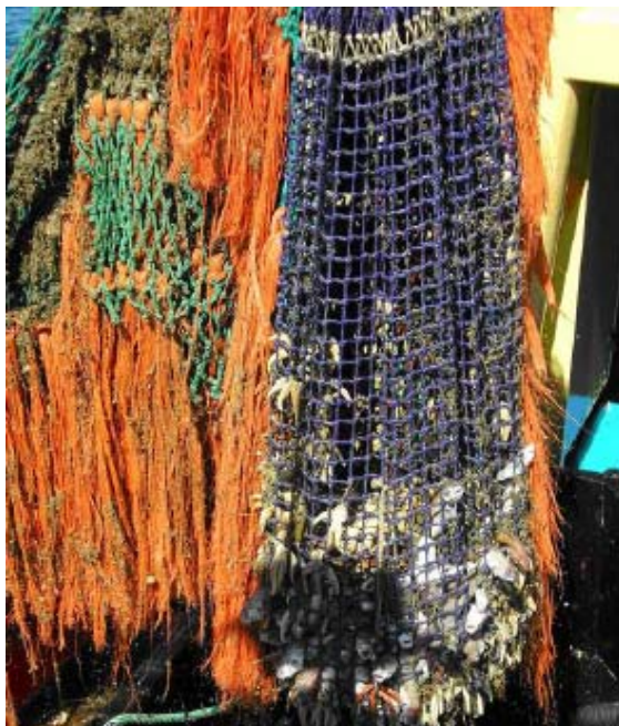
Figure 9 Square mesh cod-end being emptied on a beam trawler
