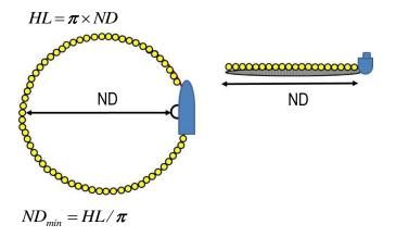
As the relationship between ND and depth has to respect the MEDREG, ND = depth/70%, HL is also linked to depth as follows:  $HL = \pi \times depth/70\%$ . Using this relationship it is possible to define the maximum feasible and allowed HL length by depth:
