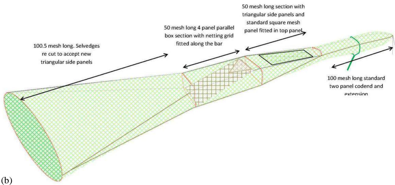
Figure 6.9.1. Net Grid modified (a) Design 1 long version; (b) design 2 short version.
