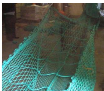
Figure 6.3.1. Large mesh upper panel of the SELTRA trawl and positioning in the trawl.
