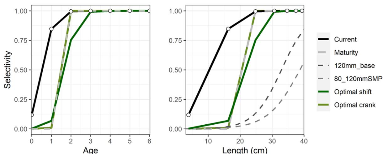
**Figure 4.5.5.2** Whiting in Division 7.a (Irish Sea) (whg.27.7a). Fitted 'Current' and 'Optimal' (shifted) selectivity by age (left) and by length (right) under current F, plotted together with the maturity ogive. Points represent the observed selectivity. Also shown on the right are gear selectivity curves for the baseline 120mm ('120mm\_baseline') and for the 80mm codend with 120mm square mesh panel that is the main gear in the Nephrops directed fishery ('80mm\_120mmSMP').
