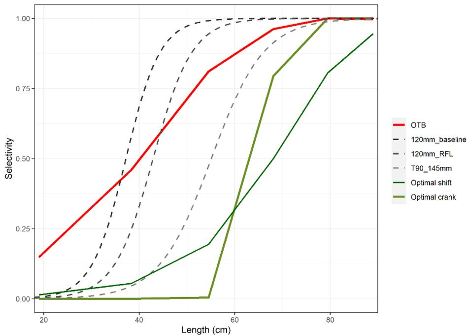
**Figure 4.5.3.4** Cod in Division 6.a (West of Scotland) (cod.27.6a). Fitted 'Optimal' selectivity by length ('Optimal shift' and 'Optimal crank'), fitted selectivity by the OTB fleet segment ('OTB'), gear selectivity curves for the baseline 120mm ('120mm\_baseline'), 120mm in a trawl with 1m raised fishing line ('120\_RFL') and a more selective alternative: 145mm T90 codend ('T90\_145mm').
