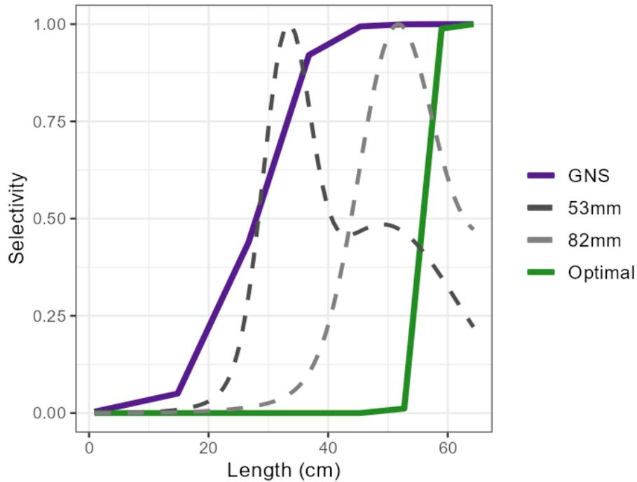
**Figure 4.6.2.5** HKE.08-09-10-11. Fitted optimal ('shift') selectivity by length ('Optimal'), fitted selectivity by the GNS fleet segment ('GNS'), gear selectivity curves for the baseline 53mm gillnet ('53mm') and a more selective 82mm gillnet ('82 mm').
