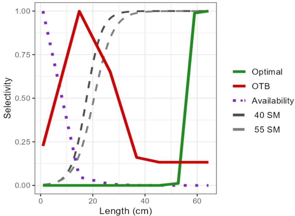
**Figure 4.6.2.4** HKE.08-09-10-11. Fitted 'Optimal' (shifted) selectivity by length, fitted selectivity by the OTB fleet segment ('OTB'), gear selectivity curves for the baseline 40mm square mesh trawler ('40 SM') and the 55mm square mesh codend trawler ('55 SM') and presumed relative 'Availability' of different sizes (inferred as the ratio 'OTB'/40 SM' scaled to 1), assuming total and unbiased implementation of the 40SM by the OTB fleet segment.
