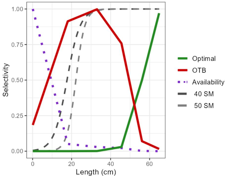
**Figure 4.6.1.4** HKE.01-05-06-07. Fitted 'Optimal' (shifted) selectivity by length, fitted selectivity by the OTB fleet segment ('OTB'), gear selectivity curves for the baseline 40 mm square mesh trawler ('40 SM') and the 50 mm square mesh codend trawler ('50 SM') and presumed relative 'Availability' of different sizes (inferred as the ratio 'OTB'/Gear 40 SM' scaled to 1), assuming total and unbiased implementation of the 40 SM by the OTB fleet segment.
