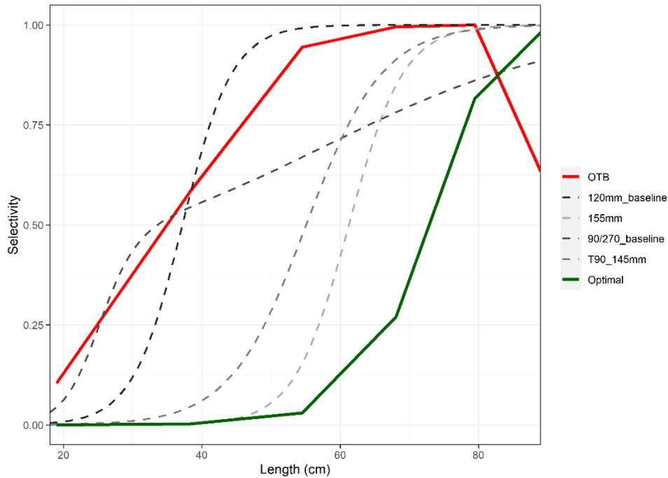
**Figure 4.5.2.4** Cod in Subarea 4, Division 7.d, and Subdivision 20 (cod.27.47d20). Fitted 'Optimal' (shifted) selectivity by length ('Optimal'), fitted selectivity by the OTB fleet segment ('OTB'), gear selectivity curves for the baseline 120mm ('120mm\_baseline'), the Skagerrak baseline 90mm with 270mm window ('90/270\_baseline') and two more selective alternatives: 155mm codend ('155mm') and 145mm T90 codend ('T90\_145mm').
