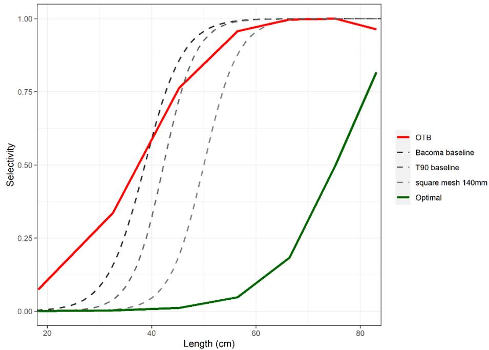
**Figure 4.5.1.4** Cod in subdivisions 22–24, western Baltic stock (cod.27.22-24). Fitted 'Optimal' (shifted) selectivity by length, fitted selectivity by the OTB fleet segment ('OTB'), gear selectivity curves for the baseline 120 mm T90 ('T90 baseline'), the baseline 105 mm with 120 mm square mesh window ('Bacoma baseline') and a more selective alternative: 140 mm square mesh codend ('square mesh 140mm').
