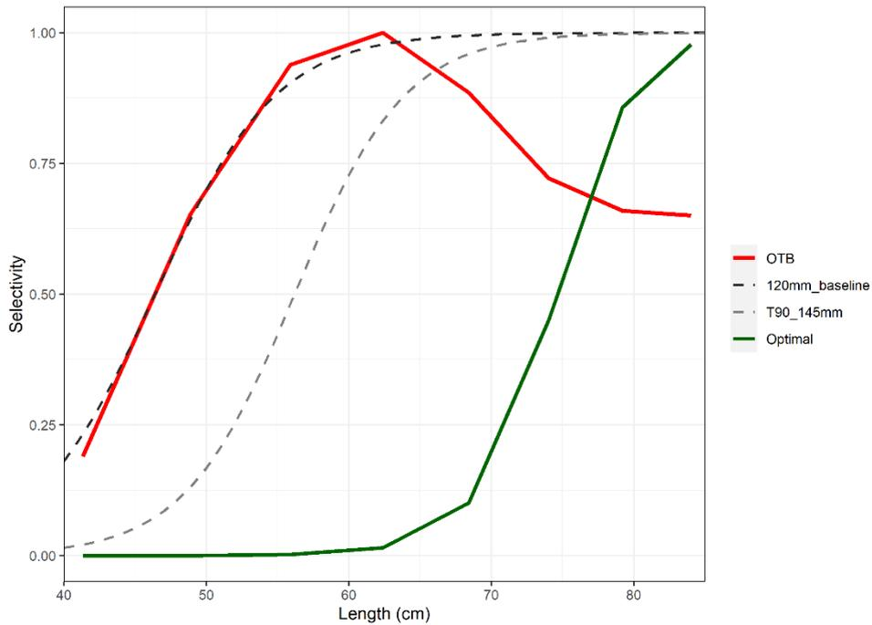
**Figure 4.5.6.4** Saithe in subareas 4 and 6, and in Division 3.a (North Sea, Rockall and West of Scotland, Skagerrak and Kattegat) (pok.27.3a46). Fitted 'Optimal' (shifted) selectivity by length, fitted selectivity by the OTB fleet segment ('OTB'), gear selectivity curves for the baseline 120mm ('120mm\_baseline') and a more selective alternative 145mm T90 codend ('T90\_145mm').
